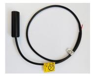
Laser pointer consisting of a high quality 635 nm red light laser diode with 1mW power. The pointer generates a very sharp and precise cross with a thickness of 1mm on black, focused at 200mm.
